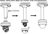
Figure 2-14 Finish Installation
