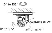
Figure 2-4 3-Axis Adjustment
