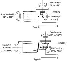
Figure 2-32 3-axis Adjustment
